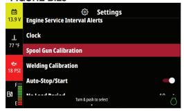
Step 3: The calibration process will feed wire out of the spool gun for several seconds. Press the knob to start the wire feeding.
