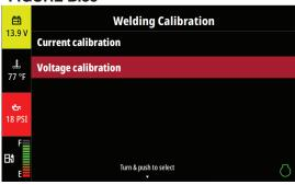
Using the knob adjust your voltage to the desired value. Press the knob to turn on your output.
