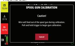
Step 2: Load the desired wire into the spool gun. Feed wire out of gun and then trim it flush with the contact tip. Press the knob to continue.
