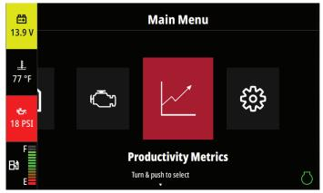
The Productivity Metrics screen provides information and statistics on how the machine is being utilized. Five statistics are monitored:
