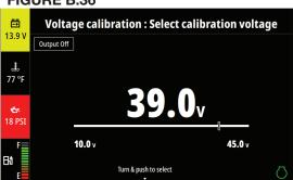
Using the knob adjust your trimmer value until your displayed and measured voltage match. Press the knob to accept the new value.
