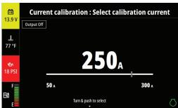
Using the knob adjust your trimmer value until your displayed and measured current match. Press the knob to accept the new value.
