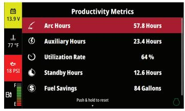
In order to reset any of these metrics, rotate the knob until the desired item is highlighted in red. Then, press and hold the knob on the selected parameter for 5 seconds.
