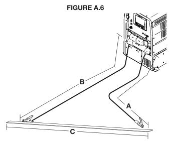
To minimize inductance always use the appropriate size cables, and whenever possible, run the electrode and work cables in close proximity to one another to minimize the loop area. Since the most significant factor in cable inductance is the welding loop length, avoid excessive lengths and do not coil excess cable. Excess cable should be placed in a straight or zig-zag pattern between the machine and work per Figure A.7.
