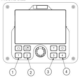
To save a memory, hold the desired memory button until the screen indicates that the memory has been saved.
