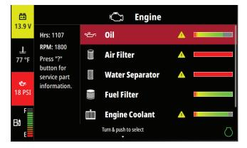
The status bars are based off the recommended service intervals and indicate the remaining time before service is required. A warning indicator will appear if a service item is nearing the end of its service life. The default warning threshold is 10%. The threshold can be configured in the SETTINGS menu.
