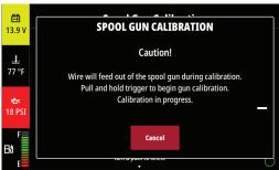
Step 5: Rotate the knob to adjust the value shown on the screen to match the actual measured length of wire. Press the knob to complete spool gun calibration.
