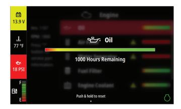
After service has been performed on an item, select it from the list and press and hold the knob for 5 seconds to reset the service indicator.
