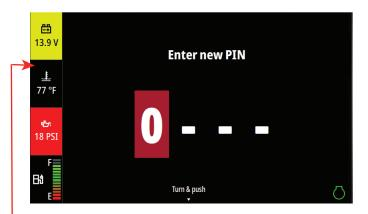
OPERATOR SECURITY - When the Operator PIN is enabled, the user interface will be locked and the generator output will be disabled until the proper PIN has been entered. A time delay may be entered that will allow the user interface to remain unlocked and the machine to be restarted throughout the day without needing to reenter the PIN.
